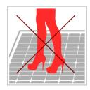
do not stand and walk on the module if it is not placed on a flat and fine surface, without visible faults, elevations and curves
